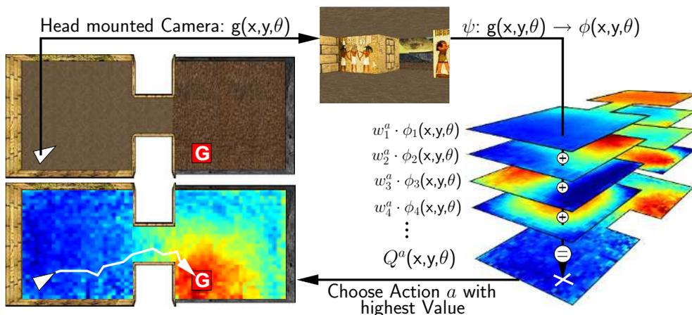
Figure 1: *Navigation control*: The robots view (interpreted as current state) is mapped into a feature space suitable for linear Q-value approximation. The action with highest Q-value is selected until the rewarded goal area **G** is reached.
